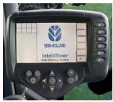
The New Holland  $VT^{\mathsf{TM}}$  colour monitor provides complete interface with the IntelliSteer  $^{\mathsf{TM}}$  system.
